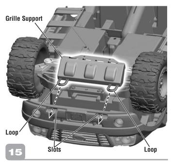
• Fit the loops on grille support through the slots in the grille. Push to **"snap"** the loops in place.
